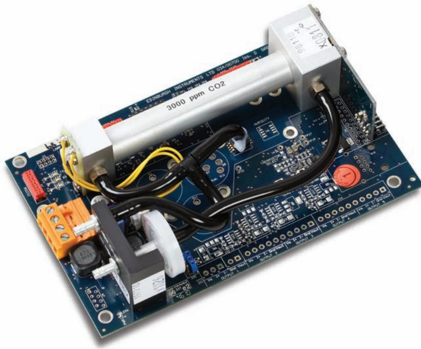
The OEM Gascard® NG infrared gas sensor, supplied by Edinburgh Sensors has been designed for easy integration into a wide range of gas detection systems where high quality, long term stability, excellent repeatability and reliable measurement of Carbon Dioxide, Carbon Monoxide and Methane gas concentrations are required.
